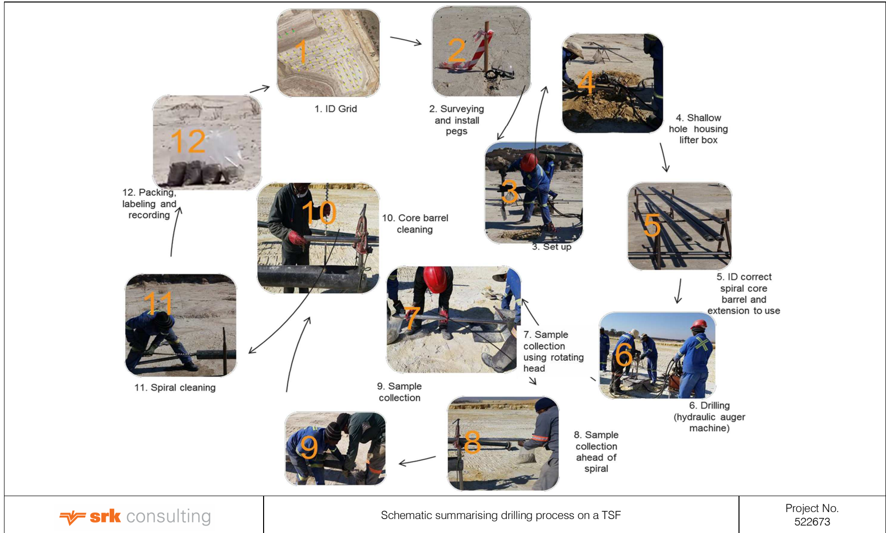
Figure 3.2: Schematic summarising drilling process on a TSF
