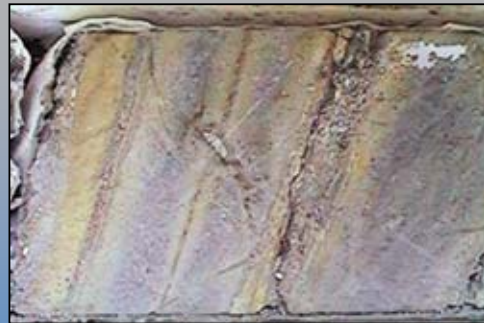
343.4m: 2m @ 27.6 g/tAu. Siltstone & veinlets with bleached margins overprinted by very fine silica/pyrite.
