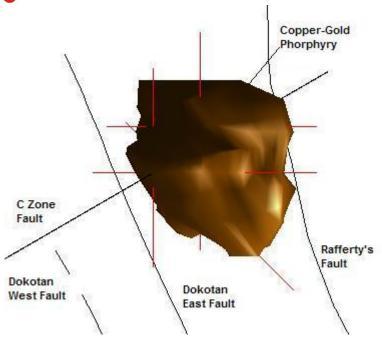
Golpu plan view showing major structures and geotechnical drilling program planned holes
