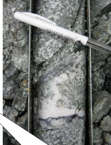
APDH001 : 466m @ 2.36g/t Ag from 17m; 59m @ 2.04g/t Ag, 0.16% Pb, 0.3% Zn from 521m. Veined and altered granodiorite containing base metal mineralisation (galena and sphalerite)
