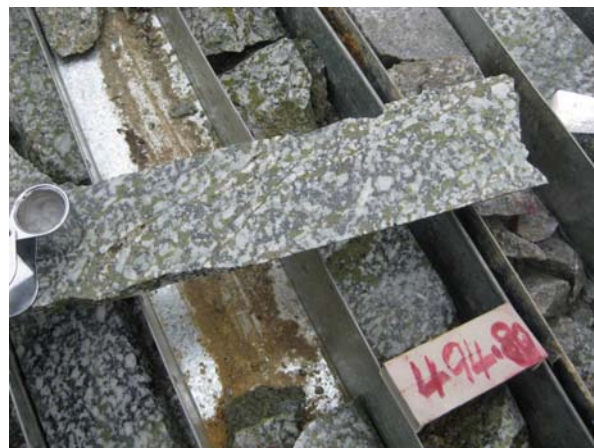
APUDH01: Strong pervasive epidote alteration at 494m
