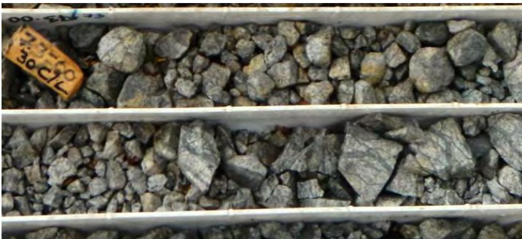
KT003: veined sericite altered diorite porphyry. Interval shown 73-75m: 1.1 g/t Au, 0.6% Cu
